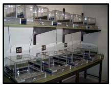
equipped with two lines of photocells at different heights, this system allows for automated recording of horizontal and vertical movement, as well as stereotyped behavior.
